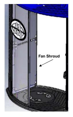
Remove the 4 black knobs from the front side of each fan shroud and remove both shrouds.
