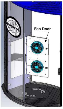
Using a screwdriver, turn the latch counter-clockwise to unlock and open the fan door.
