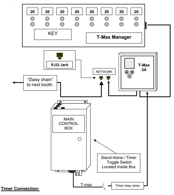
The wall mounted main control box has two inputs marked 'timer.' Connect two low voltage wires from these inputs to the timer relay wires. The Stand-Alone / Timer toggle switch must be set in the timer mode.
