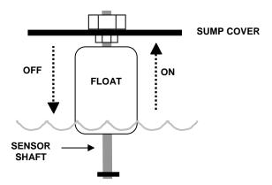
Note: When the Drain Pump float switch is in the up position, there is a 3-second delay before the Drain Pump activates.
