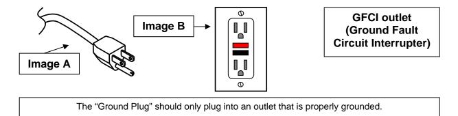
A three-prong cord and matching GFCI outlet (Ground Fault Circuit Interrupter) with a properly installed ground connection must be used with this product (see *Image A*).
